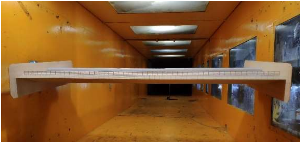
Figure 33. Free vibration wind tunnel test for flutter (1:50 scale).
